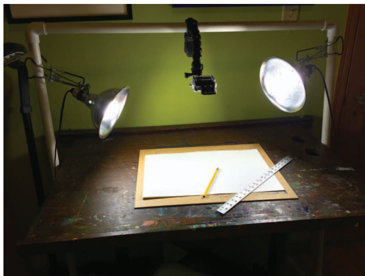
Basic studio set up for filming a drawing tutorial using a GoPro camera and studio lights clamped to a simple PVC pipe structure.
